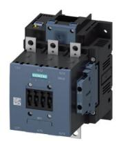
power contactor, AC-3e/AC-3 115 A, 55 kW / 400 V, AC (50-60 Hz) / DC Uc: 21-27.3 V PLC input 24 V DC 3-pole, auxiliary contacts 2 NO + 2 NC drive: electronic main circuit: busbar control and auxiliary circuit: screw terminal
