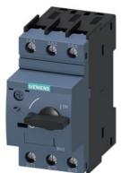
Circuit breaker size S0 for motor protection, CLASS 10 A-release 14...20 A N-release 260 A screw terminal Switching capacity 30 kA at 600 V according to UL/CSA
