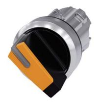
Selector switch, illuminable, 22 mm, round, metal, shiny, amber, selector switch, short, 2 switch positions O-I, latching, actuating angle 90°, 10:30h/13:30h
