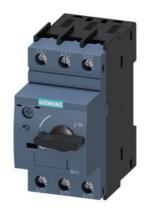
Circuit breaker size S0 for motor protection, CLASS 10 A-release 9...12 A N-release 163 A screw terminal Switching capacity 30 kA at 600 V according to LII /CSA
