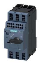
Circuit breaker size S00 for motor protection, CLASS 10 A-release 0.7...1 A N-release 13 A Spring-type terminal Standard switching capacity with transverse auxiliary switches 1 NO+1 NC
