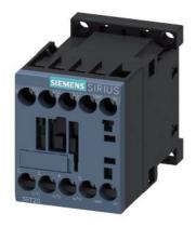
power contactor, AC-3e/AC-3, 9 A, 4 kW / 400 V, 3-pole, 110 V AC, 50 Hz / 120 V, 60 Hz, auxiliary contacts: 1 NO, screw terminal, size: S00
