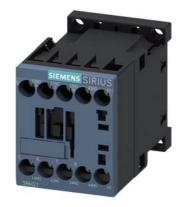
Contactor relay, 3 NO + 1 NC, 110 V AC, 50 Hz, 120 V, 60 Hz, Size S00, screw terminal
