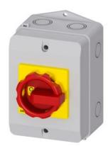
SENTRON, Switch disconnector 3LD, emergency switching-off switch, 3- pole, lu: 32 A, operating power / at AC-23 A 400 V: 11.5 kW, molded-plastic encapsulation for inch cable gland, rotary operating mechanism, red/yellow
