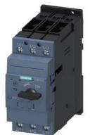
Circuit breaker size S2 for motor protection, CLASS 10 A-release 32...40 A N-release 585 A screw terminal Standard switching capacity
