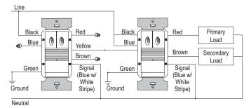
Signal wire connects to neutral. Signal wire can connect to ground in replacement or retrofit application
