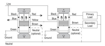
Simple optional neutral connection allows installation in any 2-wire or 3-wire application. When used in a multi-way application, all devices in that space must be wired using the same method of either with neutral
