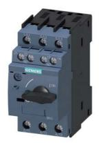
Circuit breaker size S00 for motor protection, CLASS 10 A-release 0.22...0.32 A N-release 4.2 A screw terminal Standard switching capacity with transverse auxiliary switches 1 NO+1 NC
