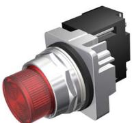
30mm Command/52, Chrome Finish Heavy Duty,Watertight/Oiltight Complete Metal Unit Illuminated Indicator Light Full Voltage type, 120V AC/DC Incandescent Lamp, BA9s Plastic Lens, Red UL Listed, CSA Certified NEMA 1,3,3R,4,4X,12,13 & Automotive Standards
