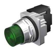
30mm Command/52, Chrome Finish Heavy Duty, Watertight/Oiltight Complete Metal Unit Illuminated Indicator Light Full Voltage type, 24V AC/DC Incandescent Lamp, BA9s Plastic Lens, Green UL Listed, CSA Certified NEMA 1,3,3R,4,4X,12,13 & Automotive Standards
