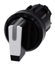
Selector switch, illuminable, 22 mm, round, plastic, white, selector switch, short, 3 switch positions I-O-II, latching, actuating angle 2x45°, 10:30h/12h/13:30h
