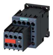
power contactor, AC-3e/AC-3, 9 A, 4 kW / 400 V, 3-pole, 24 V DC, auxiliary contacts: 2 NO + 2 NC, screw terminal, size: S00, captive auxiliary switch
