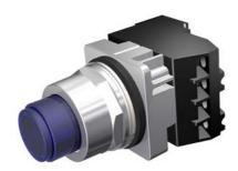
30mm Command/52, Chrome Finish Heavy Duty, Watertight/Oiltight Complete Metal Unit PTT / Illuminated Pushbutton Transformer type, 120V AC Incandescent Lamp Extended Button Plastic Lens, Blue 2 Position Momentary with 1 N.O. - 1 N.C. Heavy Duty Contacts, A600/P600 UL Listed, CSA Certified NEMA 1,3,3R,4,4X,12,13 & Automotive Standards
