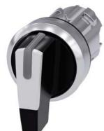
Selector switch, illuminable, 22 mm, round, metal, shiny, white, selector switch, long, 3 switch positions I>O<II, momentary contact on the left, latching on the right, actuating angle 2x45°, 10:30h/12h/13:30h
