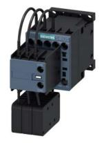
capacitor contactor, AC-6b 12.5 kVAr, / 400 V, 3-pole, 24 V DC, auxiliary contacts: 1 NO + 1 NC, screw terminal, size: S00  $\,$
