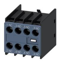
auxiliary switch, on the front, 3 NO + 1 NC, .1/.2, .3/.4, .3/.4, .3/.4, current path: 1 NC, 1 NO, 1 NO, 1 NO screw terminal, for contactors 3RT2 and contactor relays 3RH2
