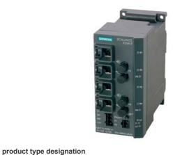
SCALANCE X204-2, managed IE switch, 4x 10/100 Mbit/s RJ45 ports, 2x 100 Mbit/s multimode BFOC, LED diagnostics, error signaling contact with set pushbutton, redundant power supply, PROFINET IO device, network management; Redundancy Manager integrated, incl. electron. manual on CD-ROM, C-PLUG optional.
