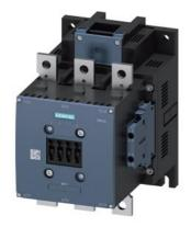
power contactor, AC-3e/AC-3 225 A, 110 kW / 400 V AC (50-60 Hz) / DC Uc: 23-26 V 3-pole, auxiliary contacts 2 NO + 2 NC drive: conventional main circuit: busbar control and auxiliary circuit: screw terminal
