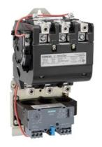
Non-reversing motor starter Size 2 1/2 Three phase full voltage Solid-state overload relay OLRelay amp range 25-100A 110-120/220-240VAC 60HZ coil Combination type No enclosure
