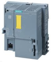
SIMATIC DP, CPU 1512SP F-1 PN for ET 200SP, central processing unit with work memory 600 KB for program and 2 MB for data, 1st interface: PROFINET IRT with 3-port switch, 25 ns bit performance, SIMATIC Memory Card required, BusAdapter required for port 1 and 2 \* \*\*\* approvals and certificates according to entry 109817615 at support.industry.siemens.com to be observed! \*\*\*\*
