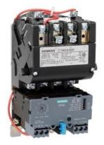
Non-reversing motor starter Size 1 Three phase full voltage Solid-state overload relay OLRelay amp range 5.5-22A 110-120/220-240VAC 60HZ coil Combination type No enclosure
