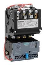
Non-reversing motor starter Size 0 Three phase full voltage Solid-state overload relay OLRelay amp range 0.75-3.4A 110-120/220-240VAC 60HZ coil Combination type No enclosure
