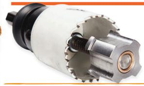
The Guide-O allows you to enlarge holes utilizing a pilot bit the same size as the existing hole. By using a pilot bit that matches up to the existing hole, the hole cutter will stay centered while drilling the new, larger hole.
