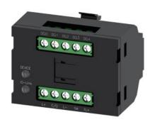
Electronics module IO-Link for ID key-operated switch, with 5 pre-programmed electronic switches, controller and RFID authentication of the switching function, black, operating voltage 24 V DC, screw terminal, for front plate mounting, for industrial application in control cabinets and machines
