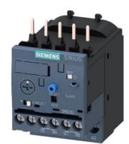
Overload relay 0.1...0.4 A Electronic For motor protection Size S00, Class 10E Contactor mounting Main circuit: Screw Auxiliary circuit: Screw Manual-Automatic-Reset
