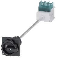
SENTRON, Switch disconnector 3LD, main switch, 3-pole, lu: 25 A, Operating power / at AC-23 A at 400 V: 9.5 kW, floor mounting with door coupling, rotary operating mechanism, black, 4-hole mounting of the handle
