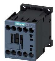
power contactor, AC-3e/AC-3, 9 A, 4 kW / 400 V, 3-pole, 24 V DC, auxiliary contacts: 1 NO, screw terminal
