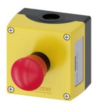
Enclosure for command devices, 22 mm, round, Enclosure material plastic, Enclosure top part yellow, 1 control point plastic, Control point in center, A=EMERGENCY STOP mushroom pushbutton red, 40 mm, rotate-tounlatch, 1 NC, screw terminal, floor mounting, 1xM20 each on top and bottom
