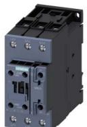
power contactor, AC-3e/AC-3, 41 A, 18.5 kW / 400 V, 3-pole, 110 V AC, 50 Hz / 120 V, 60 Hz, auxiliary contacts: 1 NO + 1 NC, screw terminal
