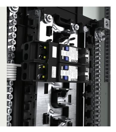
**Note:** Tandem AFCI breakers without the rejection feature can be installed in any panel that lists this specific breaker type or where a substitution letter exists for that breaker type. The schematic located on the wiring diagram will show the positions where these breakers can be placed by showing two circuits per space. The total circuits listed for panel should not be exceeded.
