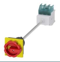
SENTRON, Switch disconnector 3LD, emergency switching-off switch, 3-pole, Iu: 32 A, operating power / at AC-23 A 400 V: 11.5 kW, floor mounting with door coupling, rotary operating mechanism, Red / yellow, 4-hole mounting of the handle, without tolerance compensation
