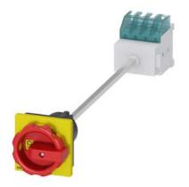
SENTRON, Switch disconnector 3LD, emergency switching-off switch, 3-pole, lu: 16 A, operating power / at AC-23 A 400 V: 7.5 kW, floor mounting with door coupling, rotary operating mechanism, Red / yellow, 4-hole mounting of the handle, without tolerance compensation
