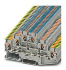
Ground modular terminal block, nom. voltage: 500 V, nominal current: 20 A, connection method: Push-in connection, 1st, 2nd and 3rd level, Rated cross section: 2.5  $mm^2$ , cross section: 0.14  $mm^2$  - 4  $mm^2$ , mounting type: NS 35/7,5, NS 35/15, color: gray
