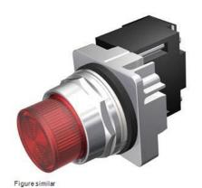
30mm Command/52, Chrome Finish Heavy Duty, Watertight/Oiltight Complete Metal Unit Illuminated Indicator Light Full Voltage type, 24V AC/DC Incandescent Lamp, BA9s Plastic Lens, Red UL Listed, CSA Certified NEMA 1,3,3R,4,4X,12,13 & Automotive Standards
