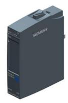
SIMATIC ET 200SP, ANALOG INPUT MODULE, AI 4XU/I 2-WIRE STANDARD, PACKING UNIT: 1 PIECE, FITS TO BU-TYPE A0, A1, COLOR CODE CC03, MODULE DIAGNOSIS, 16BIT, +/-0,3%
