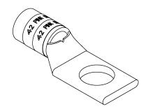
WIRE SIZE: 1/0 MATERIAL: HIGH CONDUCTIVITY COPPER
