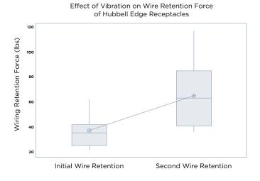
Upon installation, a 10 AWG THHN stranded wire required 40 lbs of force to disengage.
