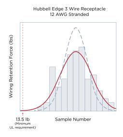
When compared to the minimum requirement for wire retention, Twist-Lock Edge screwless termination offers superior strength.
