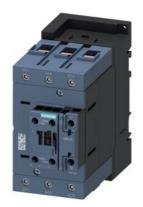
Contactor, AC-3, 55 kW/400 V 1 NO+1 NC, 110 V AC/50 Hz 120 V/60 Hz 3-pole, 3 NO, Size S3 Screw terminal
