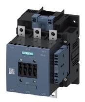
power contactor, AC-3e/AC-3 150 A, 75 kW / 400 V AC (50-60 Hz) / DC Uc: 23-26 V 3-pole, auxiliary contacts 2 NO + 2 NC drive: conventional main circuit: busbar control and auxiliary circuit: spring-loaded terminal
