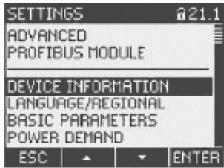
Example of operating menu: The texts can be displayed in several languages, which can be selected directly on the device.<sup>2)</sup> The large graphic LCD display facilitates reading even from a distance. For optimum visibility even in poor light conditions, the PAC4200 comes with a gradually adjustable background illumination
