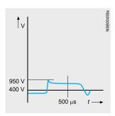
The advantages of the RC circuit lie mainly in the reduction in the rate of rise and in its RF damping ability. The selected values ensure effective interference suppression over a wide range.
