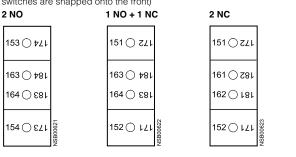
Accessories for size S3 to S12 contactors Terminal designations acc. to DIN 46 199 Part 5
