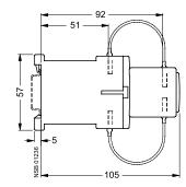
3RT16 27 capacitor contactors Size S0
