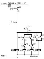
Contact element 17/18 is only closed on the star step; the contact element is open on the delta step and when de-energized.
