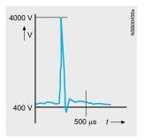
The connection between the main conducting path and the EMC interference suppression module enables contact arcing, which is responsible for contact erosion and the majority of clicking noises, to be reduced; this in turn is conducive to an electromagnetically compatible design.
