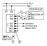
Electronics module of 3RT1 ...-.P contactor
