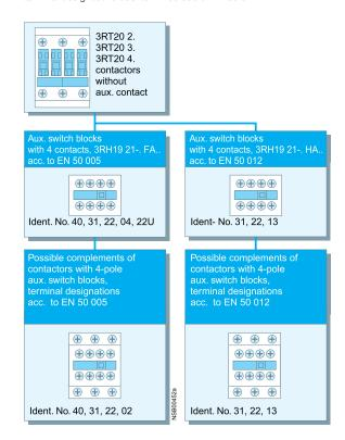
The laterally mountable auxiliary switch blocks to EN 50 012 can only be used if no 4-pole auxiliary switch blocks are snapped onto the front. If single-pole auxiliary switch blocks are used in addition, the location digits on the contactor must be noted.
