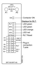
To supply power to the solenoid operating mechanism and the remaining lifetime indication, the control supply voltage  $U_{\rm s}$  must be run to terminals A1/A2 of the laterally mounted electronics module. The control inputs of the contactor are brought out to a 7-pole plug-in connection; the connector, using screwless spring-force technology, is included in the scope of supply.
