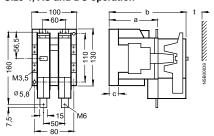
t = minimum clearance from insulated components:
