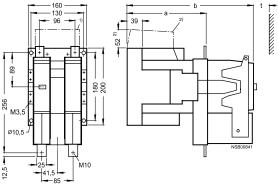
t = minimum clearance from insulated components: 25 mm (600 V and 750 V)
