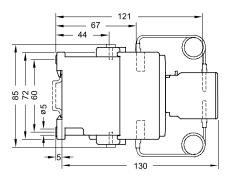
3RT16 47 capacitor contactors Size S3
