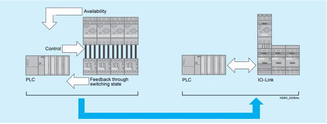
Signal transmission through IO-Link
