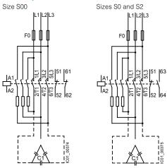
Surge suppressor (plug-in direction coded; exception: marked +/- for 3RT19 16-1T... diode assembly) for sizes S2 to S3
