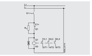
The size S00 contactors are supplied prewired with a plug-on module containing the series resistor. The suppressor diode is integrated. A 4-pole auxiliary switch block (according to EN 50005) can be fitted additionally.
