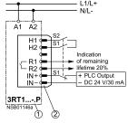
Electronics module of 3RT1 ...-.P contactor
