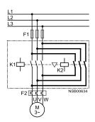
The 3RA2913-2AA. (S00) and 3RA2913-2AA (S0) installation kit contains wiring connectors for connecting the main conducting paths, the mechanical interlock and two connecting clips for the contactors.
