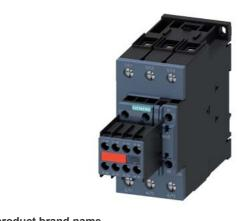
power contactor, AC-3 40 A, 18.5 kW / 400 V 2 NO + 2 NC, 110 V AC 50 Hz / 120 V, 60 Hz, 3-pole, Size S2, screw terminal captive auxiliary switch block
