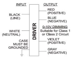
Input and output use lead-wires.
