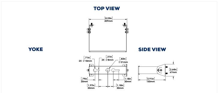
Note: Can be adjusted to increments of 30 Degrees
