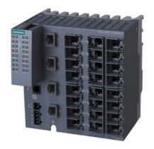
SCALANCE XC224-4C G manageable Layer 2 IE switch; IEC 62443-4-2 certified; Full gigabit; 20x 10/100/1000 Mbit/s RJ45 ports; 4x 1000 Mbit/s combo ports (either 1000 Mbit/s/ SFPs or 10/100/1000 Mbit/s RJ45 ports can be used); 1x console port; diagnostics LED; redundant power supply; temperature range -40 °C to +70 °C; assembly: DIN rail/S7 mounting rail/wall; redundancy functions; office features (RSTP, VLAN,...); PROFINET IO device; Ethernet/IP-compliant; C-PLUG slot;
