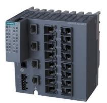
SCALANCE XC216-4C G manageable Layer 2 IE switch; IEC 62443-4-2 certified; Full gigabit; 12x 10/100/1000 Mbit/s RJ45 ports; 4x 1000 Mbit/s combo ports (either 1000 Mbit/s/ SFPs or 10/100/1000 Mbit/s RJ45 ports can be used); 1x console port; diagnostics LED; redundant power supply; temperature range -40 °C to +70 °C; assembly: DIN rail/S7 mounting rail/wall; redundancy functions; office features (RSTP, VLAN,...); PROFINET IO device; Ethernet/IP-compliant; C-PLUG slot;
