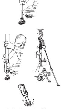
Attach anchor eye nut and the installation is complete
